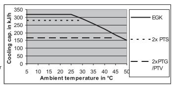
Remark: Limits shown for the heat exchangers are for an inlet dew point of 40°C.
