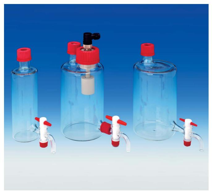
In negative pressure sample conditioning systems, condensate removal from the sample gas coolers or similar equipment requires the use of peristaltic pumps and/or of intermediate storage vessels.
