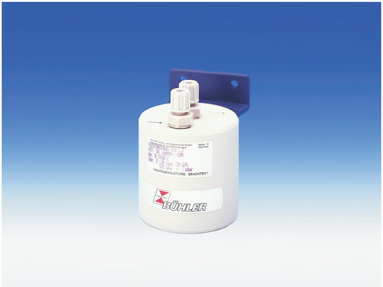
The back pressure regulator keeps the sample gas pressure constant and independent from atmospheric pressure. This avoids inaccuracies due to fluctuations in barometric pressure.
