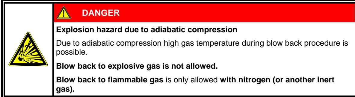
Due to adiabatic compression, high gas temperature during blow back procedure is possible. Probe with blowback are approved only for sampling non-explosive gases. Blow back of flammable gas is only allowed with nitrogen (inert gas).
